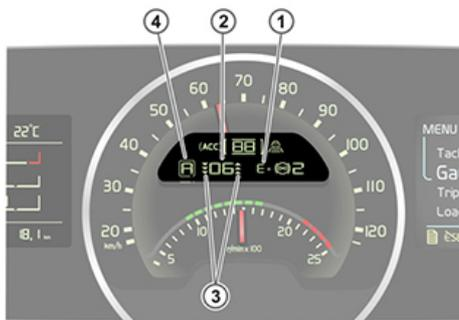
Shown in the display: 1. Driving program 2. Selected gear 3. Available gears (down/up) 4. Driving mode
